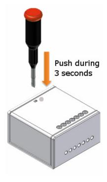
If the ZLOCK was not associated it begins flashing quickly during 20 seconds. The ZLOCK looks for a coordinator during this blinking.
