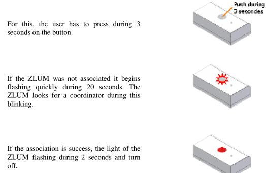
If the light of the ZLUM does not flash after pressing on the button during 3 seconds, this means that he is already associated in a network.
