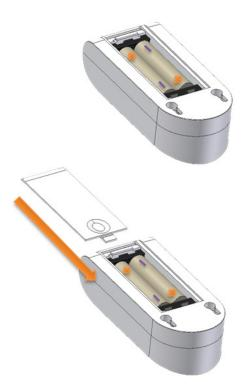
Put back the lid on the ZMETER by making it slide until it is to clip.
