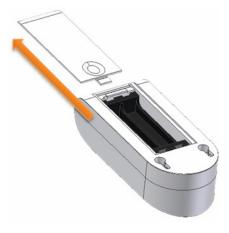
Change batteries by respecting well the indicated polarity.
