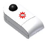
If a coordinator is present and what it authorizes the ZMOVE to join the network, the light of the ZMOVE flashing during 2 seconds then turn off.
