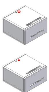
If the light of the ZXPAND does not flash after to have press on the button during 3 seconds, this means that he is already associated in a network.
