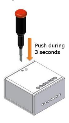
If the ZXPAND was not associated it begins flashing quickly during 20 seconds. The ZXPAND looks for a coordinator during this blinking.
